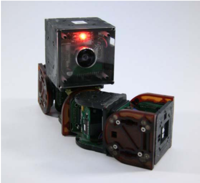
Fig. 3: One cluster of four CKbot modules with camera, battery pack, controller, and magnetic face attachments.
