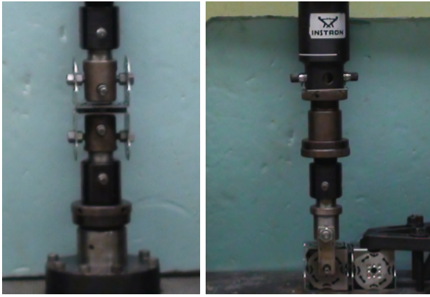
Fig. 6: Tensile (left) and bend (right) testing of the female-male ModLock element with Instron 4206
