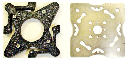
Fig. 3: Fabricated male connector plate assembly (left) and female connector pattern (right)
