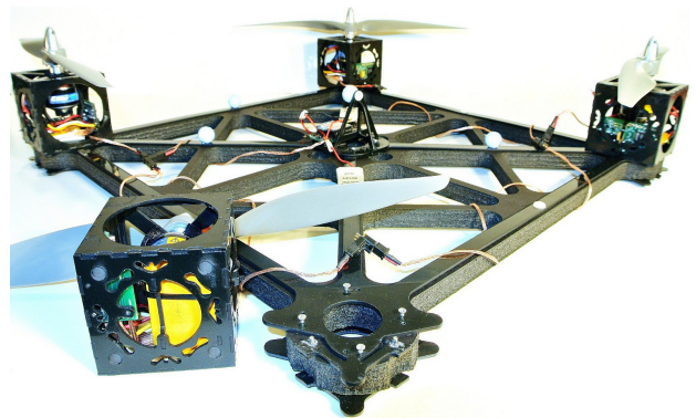
(b) Modular quadrotor with one disconnected lightweight CR module
