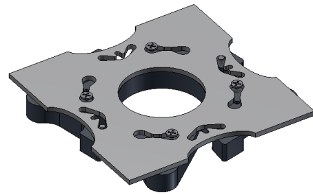
(a) Male connector plate assembly and female a pattern are pushed together
