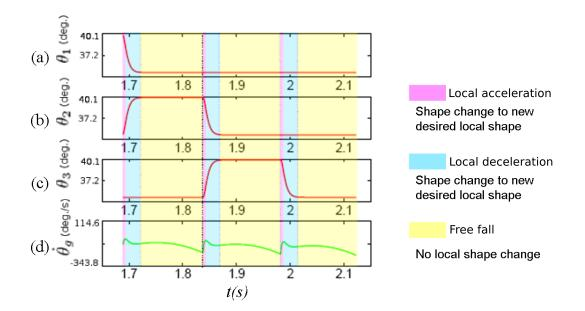
Fig. 6. Simulation results: (a) Joint angle for Module 1 (b) Joint angle for Module 2 (c) Joint angle for Module 3 (d) Angular velocity of the robot over time interval corresponding to three consecutive module touchdowns.
