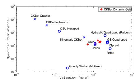
Fig. 16. Specific resistance vs. velocity for several robotic systems. The data for walking systems included here is from [Gregorio et al., 1997].
