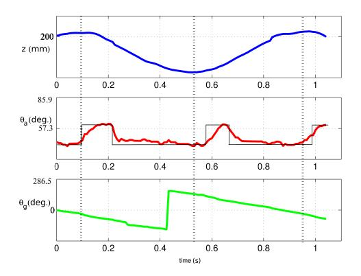
Fig. 9. Experimental results: Tracking results for one module using a motion capture system: z represents height of tracked module above the ground for one cycle,  $\alpha$  represents joint angle of tracked module,  $\alpha_g$  represents pitch of tracked module with respect to global reference frame (the discontinuity in the data is because of a jump from  $-\pi$  to  $\pi$ ).
