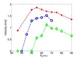
Fig. 13. Experimental results: Terminal Velocity (in m/s) vs. Apex Angle (in degrees) on  $5^{o}$  (shown with '+'),  $0^{o}$  (shown with 'o') and  $-5^{o}$  (shown with 'o') inclines.
