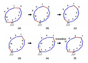
Fig. 5. Different phases of the rolling motion illustrating the effect of shape change at touchdown and subsequent falling motion of the robot. Modules change shape in (a) - (e) note apex nodes 1,6 change to 2,7 and start to pivot rigidly about node 3 (f).
