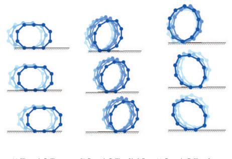
(a) Kinematic Rolling (b) Dynamic Rolling: Ideal Case (c) Dynamic Rolling: Loop turns back on itself
