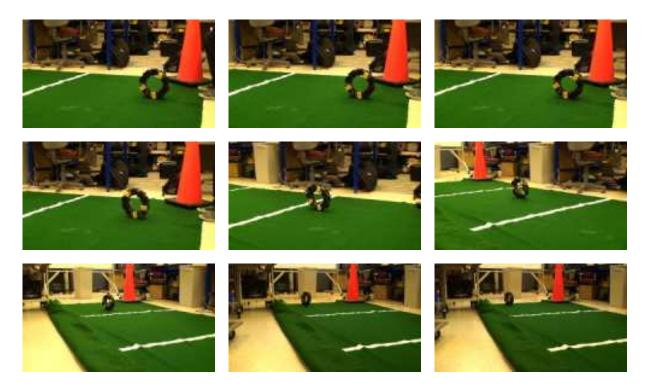
Fig. 15. Snapshots of the rolling motion. Speed was controlled by a joystick in real time. Frames are in chronological order from left to right, then top to bottom. The motion of the robot is from right to left.
